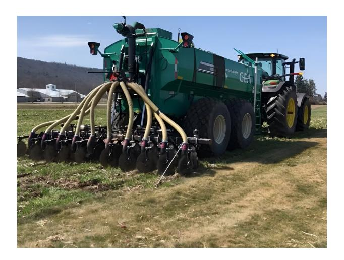
A dairy manure tanker with shallow disk injectors used for injecting liquid dairy manure into no till farm fields. Credit: Sailesh Sigdel/Penn State
