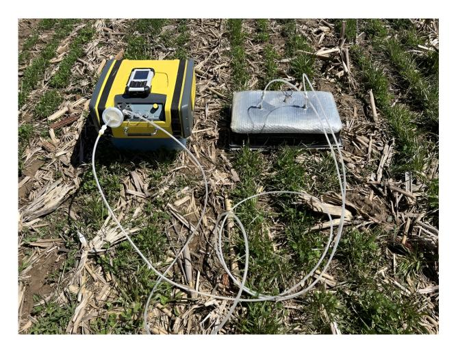
A gas analyzer connected to a vented static chamber used in this study to measure nitrous oxide emissions from a research plot. Credit: Sailesh Sigdel/Penn State
