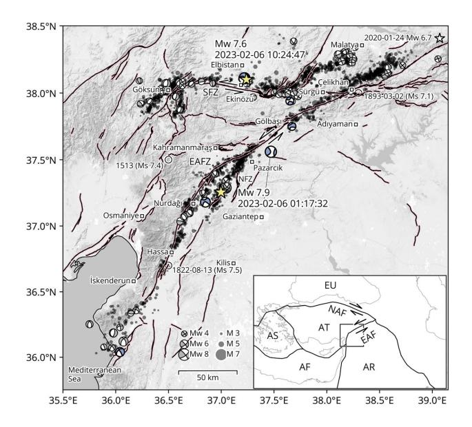
Summary of the study region. The yellow stars are the relocated epicenters of the MW 7.9 and MW 7.6 earthquakes. The dots are the relocated aftershocks
