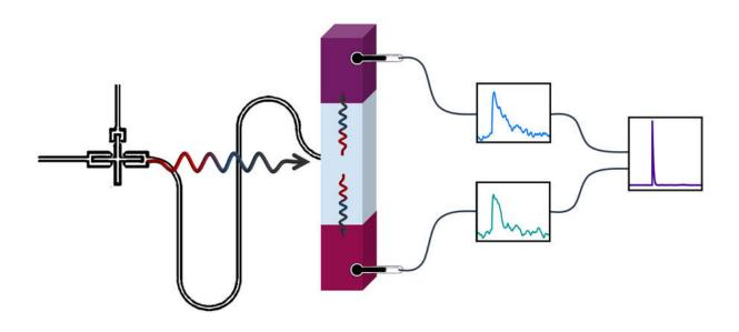
A low energy photon emitted by a qubit can potentially be detected by measuring its energy with two thermometers simultaneously. The two signals are combined into a cross-correlation measurement with superior sensitivity. Credit: Bayan Karimi
